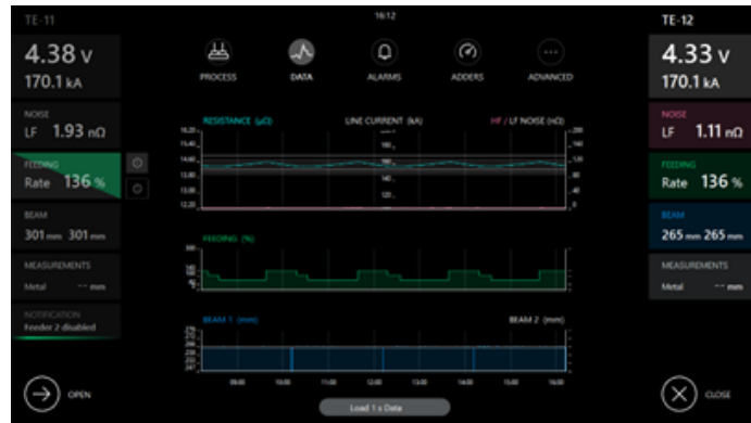
Figure 5. Hardware in the Loop (HIL) with pot simulation.
