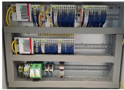
Figure 5. Hardware in the Loop (HIL) with pot simulation.
