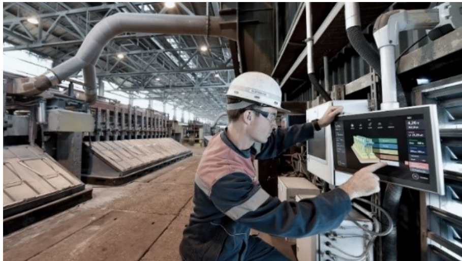
Figure 3. METRICS® L1 HMI in operation in Essen smelter.
